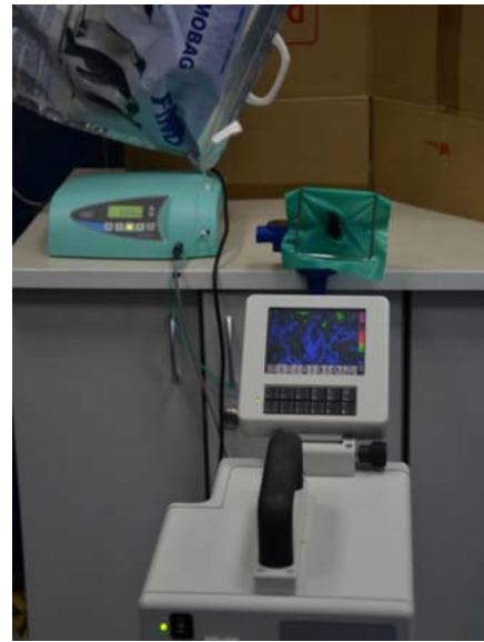
Fig. 2 – Experimental set-up – cross-sectional specimen's surface exposed to infrared camera.
